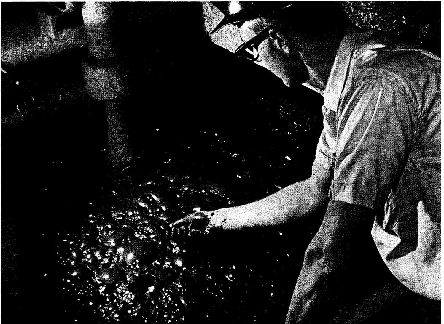
Beneath these bubbles is a swirling mixture of water, finely pulverized copper ore and various chemicals. The chemicals separate copper minerals from rock. The bubbles trap these minerals and are floated off to form a concentrate for further processing. This is one way Anaconda research is making it economically feasible to mine today's low content copper ores. It sounds simple. But it involves complex com-
